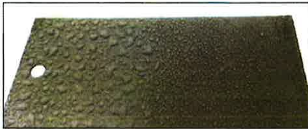
Figure 8. Panel 2 at 500 hours.
