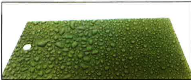
Fig. 1. Aluminum paint (Panel 1) at zero (0) hours exposure.
