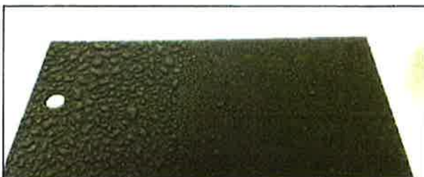
Fig. 4. Aluminum paint/Clearcoat (Panel 3) zero (0) hours.
